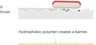
Elastomeric polymers fuse to surface.
