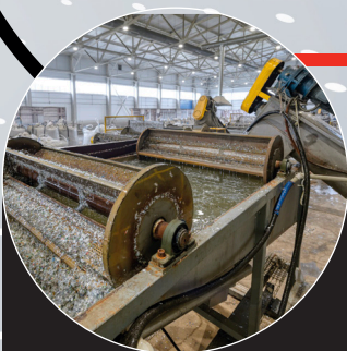
STAGE 4. Through a bathing process which separates colours.
