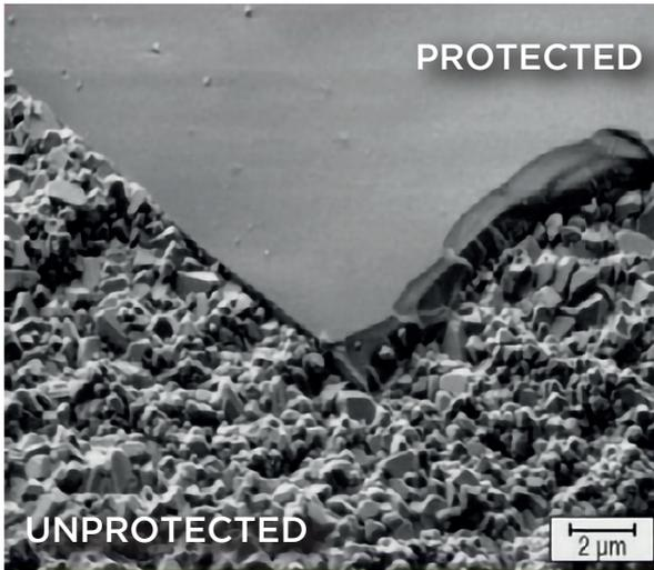
This is polysilazane under a microscope as it forms this impenetrable barrier.
